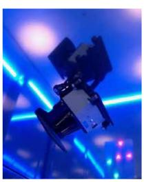
Once the owner get out from the entry cell, the system, through out some laser scanners, Will check the vehicle and his size, in order to verify they will be into the platform and avoid any car's damage, during the moving and parking process.
